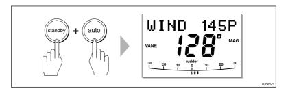
3. In Wind Vane mode, the SmartPilot will then adjust the boat's heading to maintain the locked wind angle.
